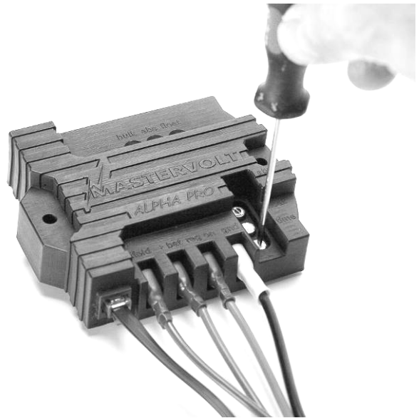
Figure 14: Adjustment of the potentiometers
