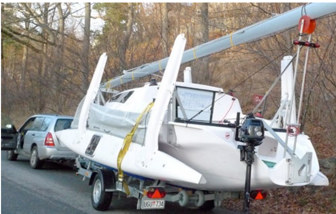
A Dash MKI showing the dagger style rudder mounted on transom. The rudder blade can be removed and stowed for transport.
