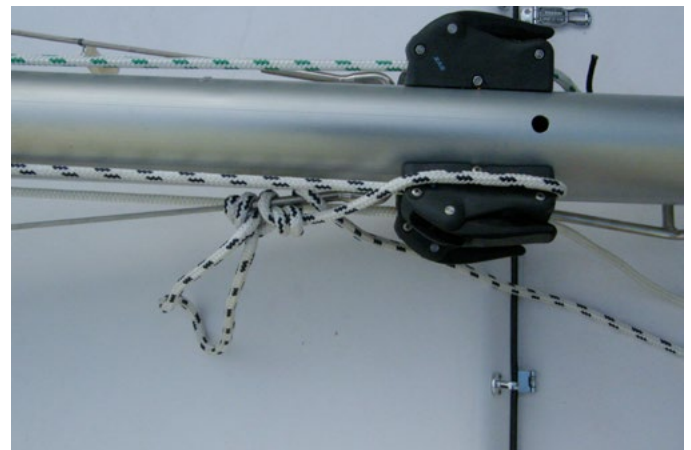
Halyard tied down as safety back up
