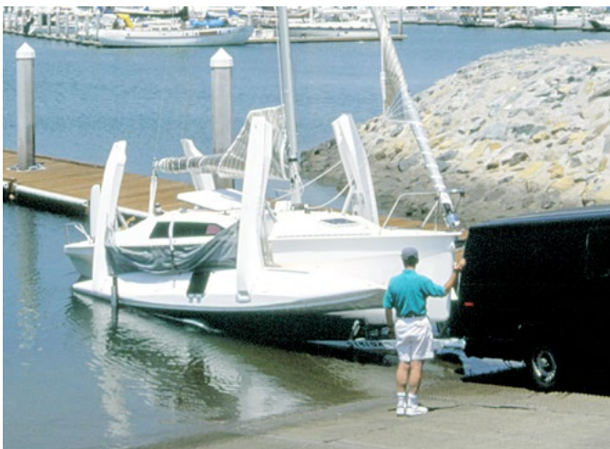
Submerge trailer to inward bend
