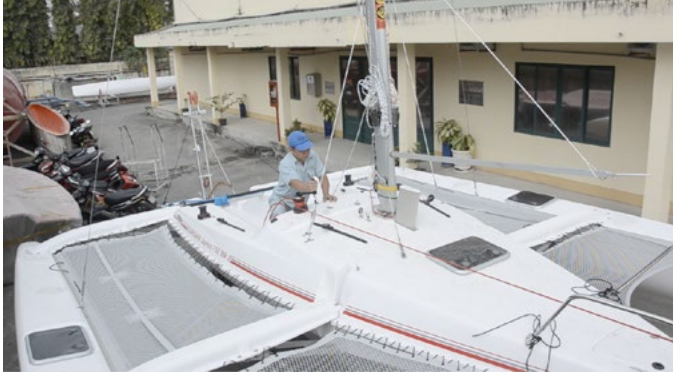
Mast on way up and being held from going sideways by raising wires
